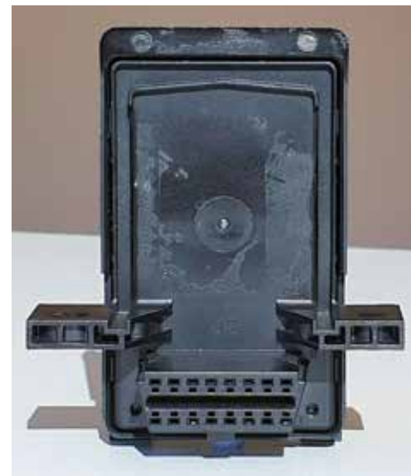
Rear view of gateway (vehicle side).
