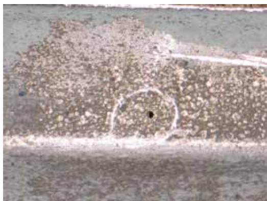
Tube cut open to show pinhole.
