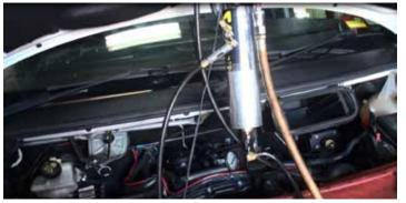
to use the correct chemical and tooling for this job. After applying a considerable amount of chemical into the turbo, it is now time to add more the induction chemical cleaner into my apparatus and then concentrate on the intake manifold side. I then set my pressure higher and continue the process.
