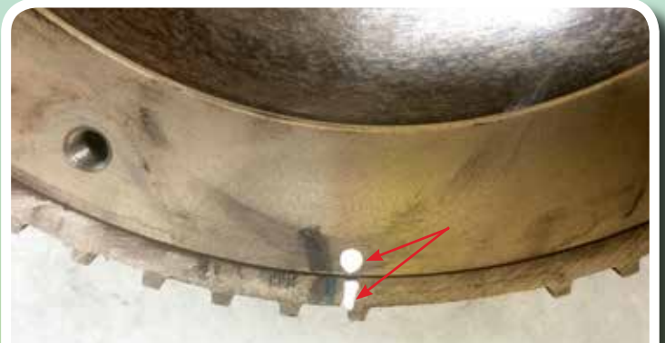
How it should have looked. Marks are aligned here. Notice the position of the missing teeth, compared to the original.
