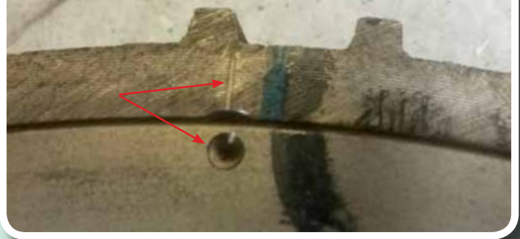
Timing mark on the flywheel & tone wheel aligned
