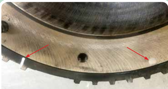
The car came in with this flywheel. Shown with white paint, the timing marks on the flywheel & tone wheel are about 50 degrees apart.
