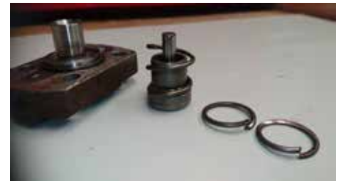
Pic shows plunger spring broken & separated
