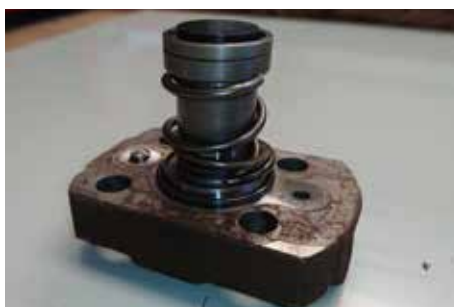
Pic shows plunger spring broken
