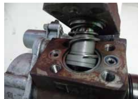
Revealed broken spring
