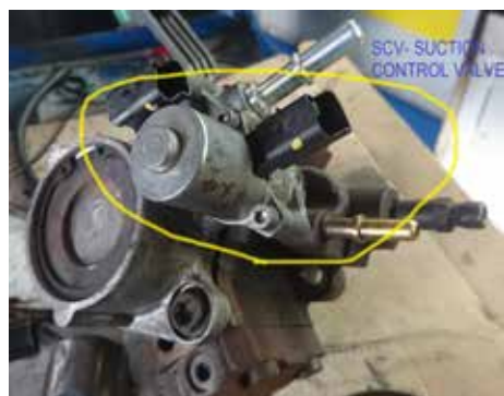
SCV location on the pump
