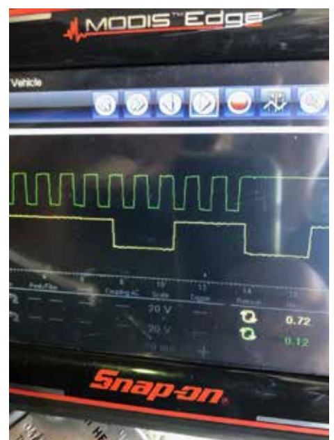
Image shows known good scope reading.
