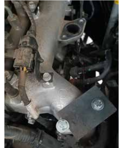
EGR connecting pipe in place EGR connecting pipe removed for testing
