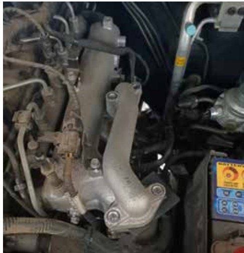
EGR connecting pipe in place EGR connecting pipe removed for testing
