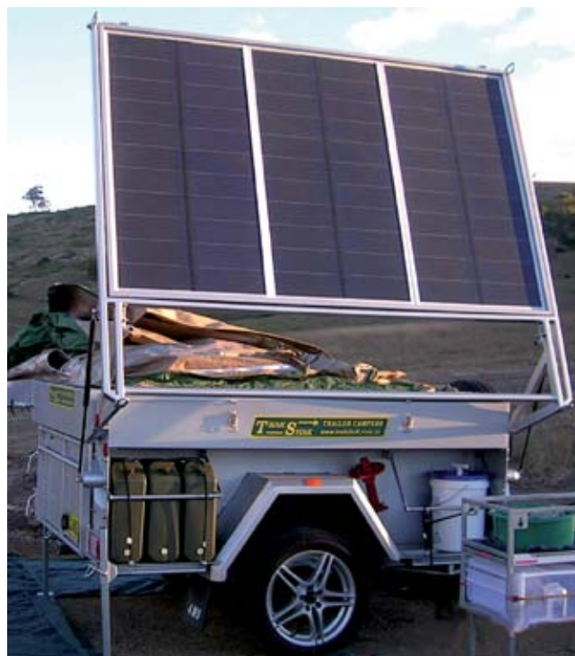
This solar modules rack is an optional extra with Track Shack camper trailers: simple and effective if the trailer is parked to face North.
