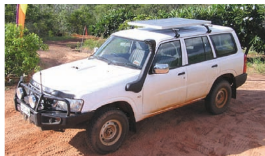
1. Author's 4.2 litre turbo diesel Nissan Patrol has two 80-watt BP solar modules charging a 100 Ah LifeLine AGM battery.
